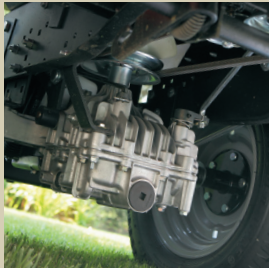
The durable Tuff Torq® transmission offers a hydrostatic drive for an automotive-like feel.
